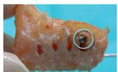
Figure 5: Distal fragment post test after removal of plate 3 showing 'long holes' and broken screw (blue circle)
