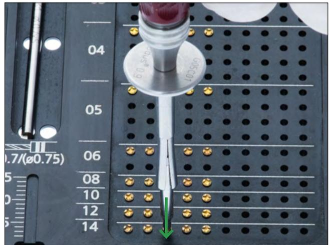
Slide the tension sleeve over the screwhead.
