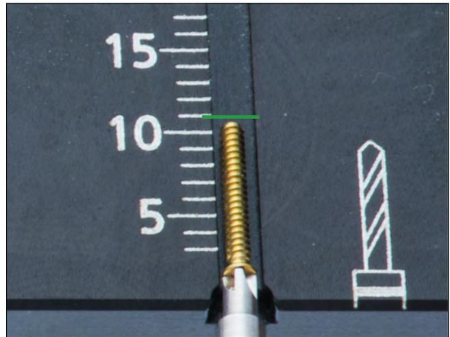
To remove the screws from the implant container using the screwdriver blade (M-2511) in combination with the tension sleeve (M-2551), insert the screwdriver blade perpendicularly into the screw head of the desired screw.
