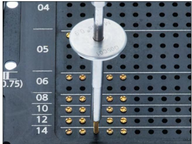
The screw length is checked with the measuring module designed for the use with the tension sleeve (M-2551).
